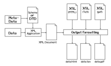
Figure 8: Preparation of XML data and examples of output formatting
