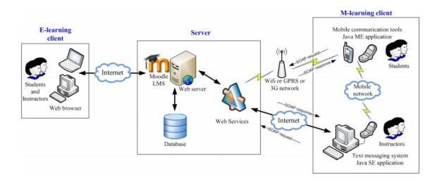
*Figure 2.* Architectural diagram of the integration of the Moodle LMS with the mobile communication tools.
